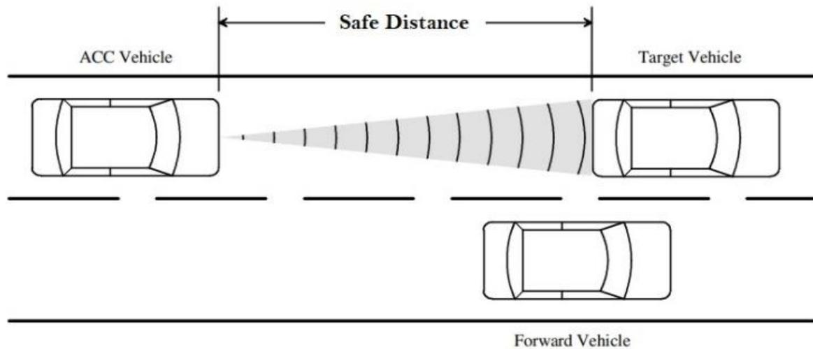
*Fig 1.1 Adaptive Cruise Control (radar application)*
