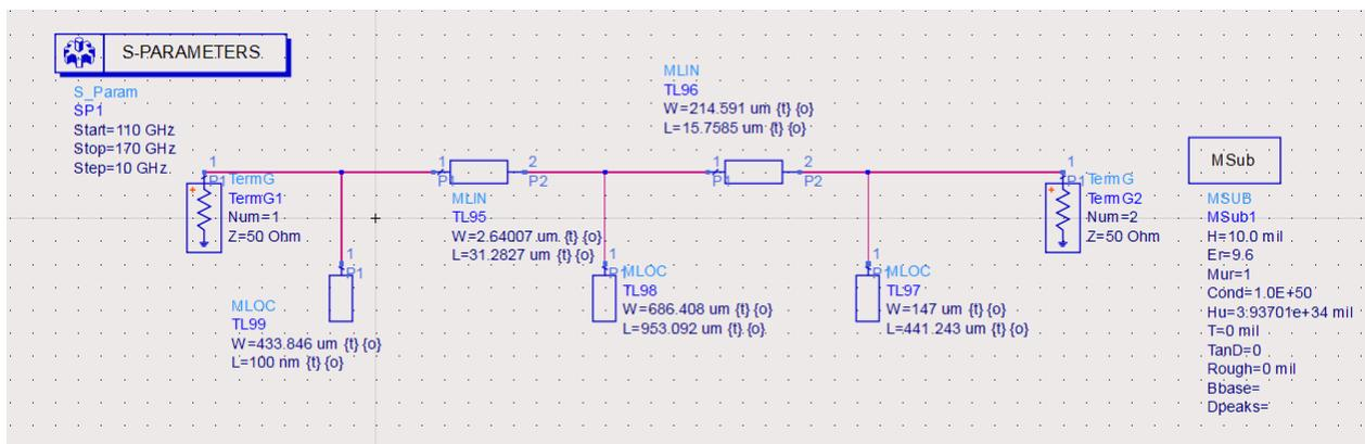
Fig 7.3.2 Intermediate matching network
