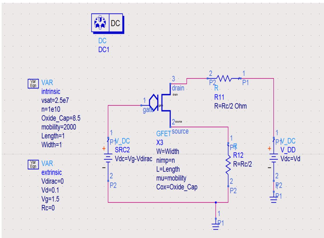
fig 7.1.a Simulation of GFET device
